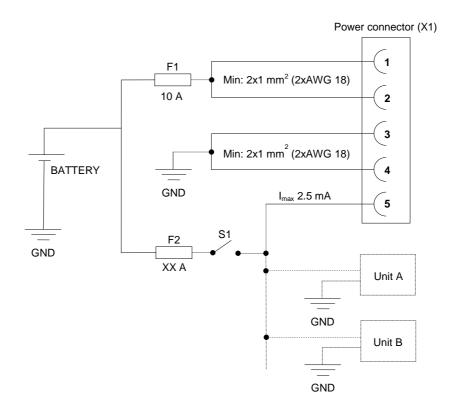
By connecting the power supply according to the illustration above, the device will automatically start when the main switch or turnkey is turned on, and shut down when the switch or turnkey is turned off. While the main switch is in the ON position, the computer can also be turned off and on with the On/Off-button. The functionality of the ON/OFF signal and On/Off button can be changed in software (CCAux API).
